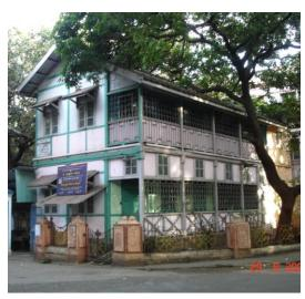
Modest scale building with timber structural members and brick filling with a road facing wooden balcony and sloping roof
