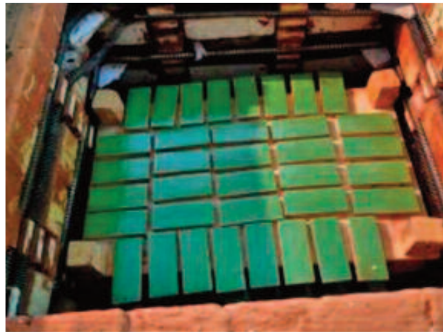
Glazed tiles in kiln after firing
